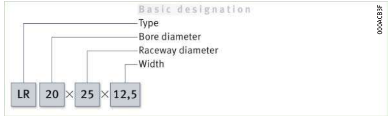
5 Inner ring LR: designation structure
